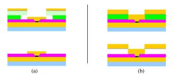
Fig. 3. Cross-section drawing of liftoff process. (a) Photoresist overhang using bilayer process makes clean pattern on substrate. (b) Lack of photoresist overhang can lead to excess metal staying on the substrate.
